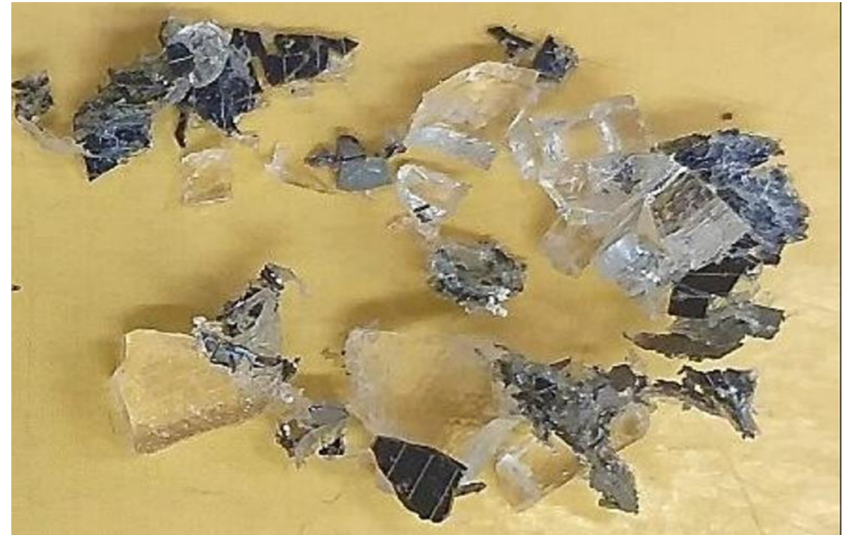
Delaminated components of a PV module employing supercritical CO 2 (Lovato et al, 2021)
