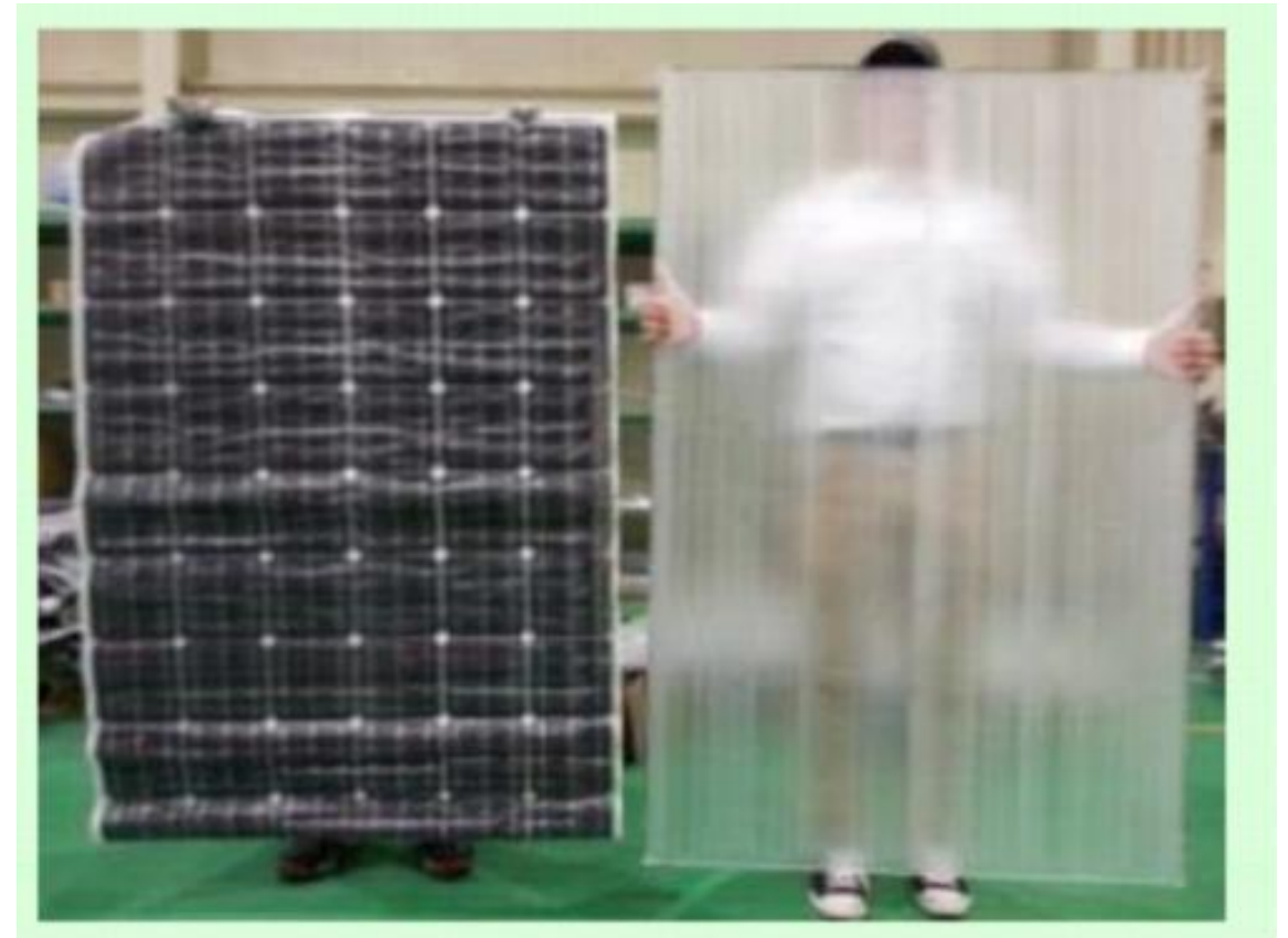
Glass separated from PV module by hot-knife technique (NPC)
